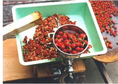
Figures 2 and 3: Illustration of a Corona grain mill, and photo of a Corona mill being used to extract the seed of a small-fruited hot pepper ('Amazzo'). The wooded "push rod" is used to force the uncut fruit into the throat of the hopper and between the threads of the auger. Small hot peppers do not need to be cored or sliced. The mash is caught in a large tray and later transferred to a bucket for fermentation. When working with small-fruited varieties, quite a bit of seed (ounces to pounds) can be extracted this way.
