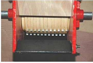
Figure 8. Throat of an apple grinder/press. Photo courtesy of Pleasant Hill Grain.
