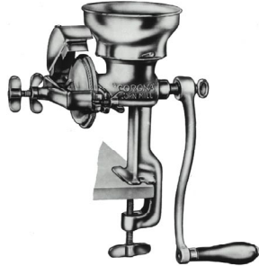
Figures 2 and 3: Illustration of a Corona grain mill, and photo of a Corona mill being used to extract the seed of a small-fruited hot pepper ('Amazzo'). The wooded "push rod" is used to force the uncut fruit into the throat of the hopper and between the threads of the auger. Small hot peppers do not need to be cored or sliced. The mash is caught in a large tray and later transferred to a bucket for fermentation. When working with small-fruited varieties, quite a bit of seed (ounces to pounds) can be extracted this way.
