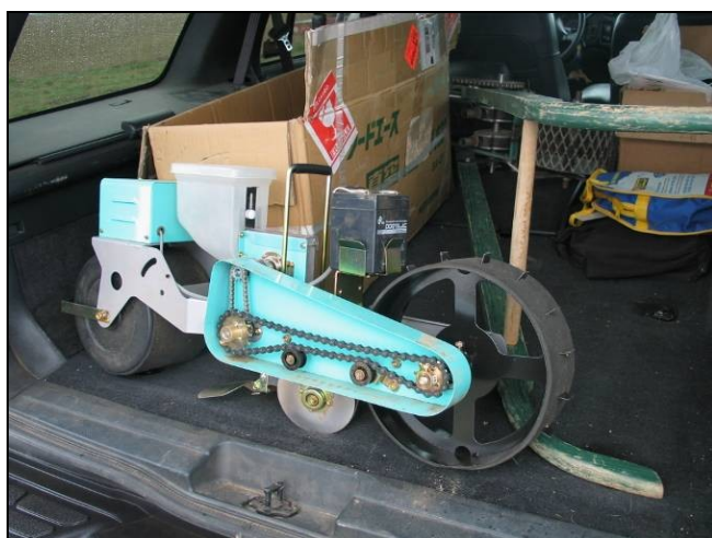
This small-scale vacuum seeder allows establishing trial plots using the same techniques as in regular production.
