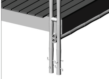
COLUMN J HOOKS AND BAMBOO BEAMS @ DECKING
